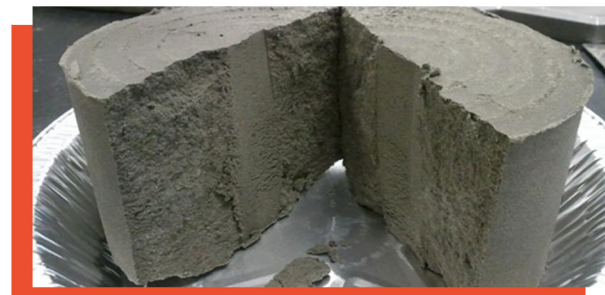
Shown here is a sample of Twin Metals tailings being tested in a lab for consistency, optimum moisture content and stability.
